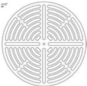
This template is a universal marking guide and cut-out stencil used for marking the center of a down-light, vent, speaker, or any hole that needs to be marked and cut in an ISC Panel.
