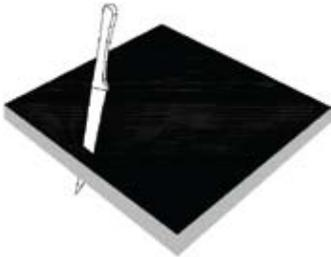
If necessary, cut the border with knife. Make sure to cut the Drop-In Panel from the face side along the marked lines. Make sure to make your cuts straight up and down and not at an angle.
