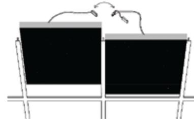
Connect a Jumper Cable to the first panel and connect it to the next panel. Up to 50 ISC Panels can be connected together in any configuration. If
